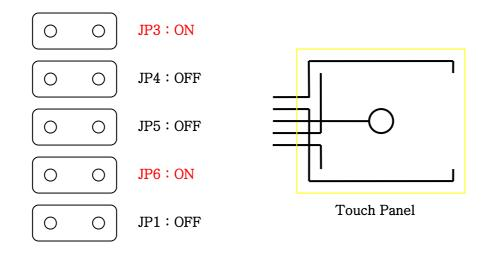
B. 3M Type Pin Assignment (When Elo driver is used)
